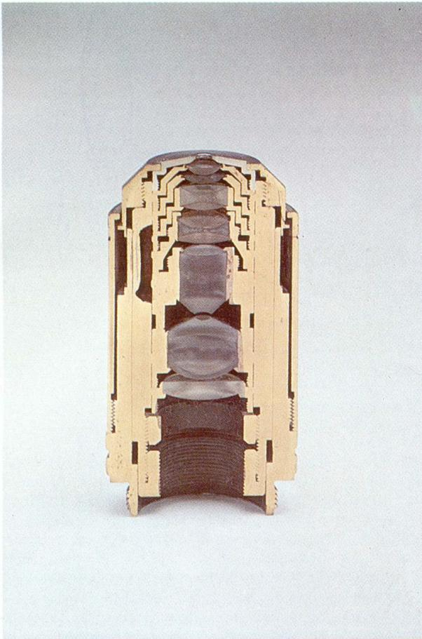
Fig. 1: Cross section through a modern plan-apochromatic LEITZ objective.
